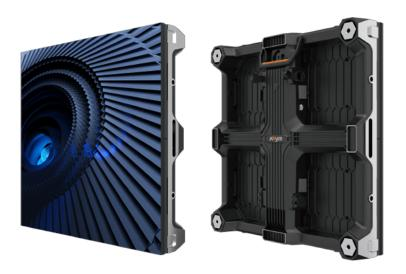
The MR series adopts the two-in-one integrated design of the cabinet and the frame, which makes the panel thinner and lighter, and the floor screen can be built without adding sub-frames at the bottom. The height of the panel can be adjusted by the anchors in case of the rough ground and the adjustable height is 0~20mm.
