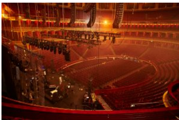
The L-ISA system, which comprised a frontal 15 system with additional Kara side hangs, X8 and SB18 as front fill, and X8 as fill for the stalls, worked 'fantastically' for FOH engineer, Adam Rhodes. Copyright James Adams
